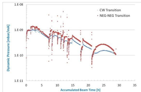
Figure 1: dynamic pressure increase in the Cold-Warm (CW) transition area and in the NEG-NEG area as a function of the beam accumulated time.
