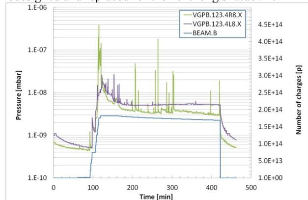
Figure 3: Pressure spikes on the vacuum RF insert modules.
