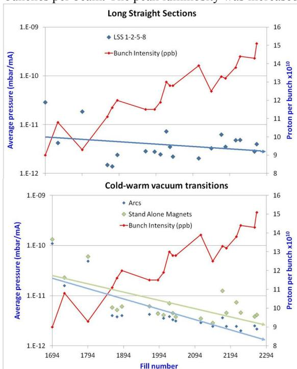
Figure 2: Overview of the average dynamic pressures in the LHC during the year 2011
