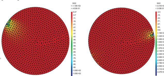
Figure 7: Principal stress field in the disc during the acceleration and deceleration phases.
