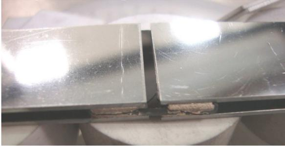
Figure 5: Brazing test of glassy carbon on metals.
