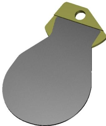
Figure 1: Dovetail connection between the glassy carbon blade and the titanium support.
