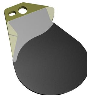
Figure 4: Dovetail connection between the glassy carbon blade and the titanium support.
