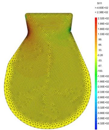
Figure 2: Principal stress field in deceleration for the dovetail geometry.
