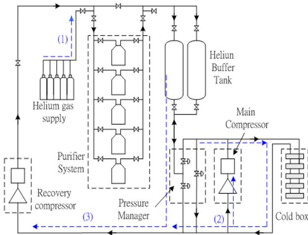
Figure 4: Configuration of the purifier system.
