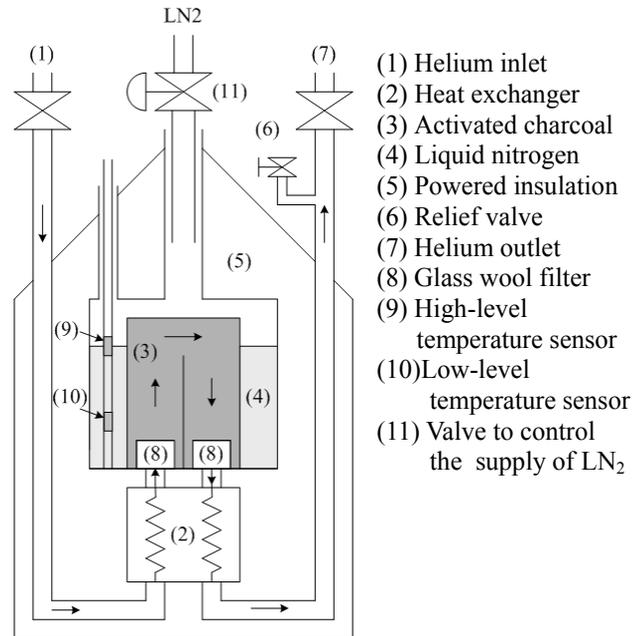
Figure 2: Cryogenic adsorber.
