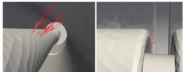
Figure 6: Multipacting at 110 kW in the coaxial line (left) and between the window and choke at 60 kW (right).
