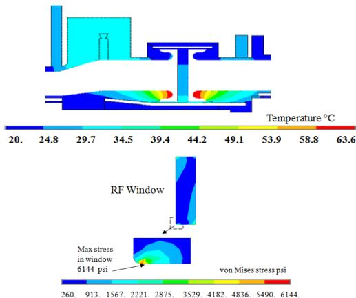
Figure 3: Temperature contours on the RF window area (top) and Von Mises stress contours (bottom) with 1MW power transmitted through.
