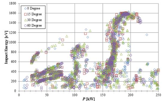
Figure 5: Multipacting simulation at different phases.
