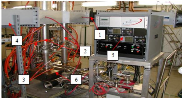
Figure 7: Assembly of the FPCs for conditioning: 1 – waveguide connecting to 1 MW klystron, 2 – two FPCs, 3 – cooling hoses, 4 – waveguide phase shifter and a short plate, 5 - vacuum instrument on the conditioning cart, 6 – connecting waveguide.
