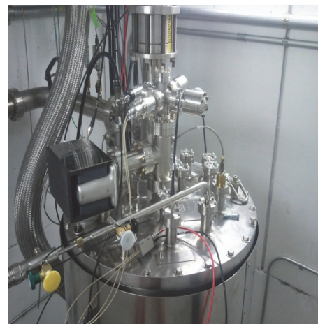
Figure 6: The large grain cavity (top) and the top plate assembly for the test (bottom).
