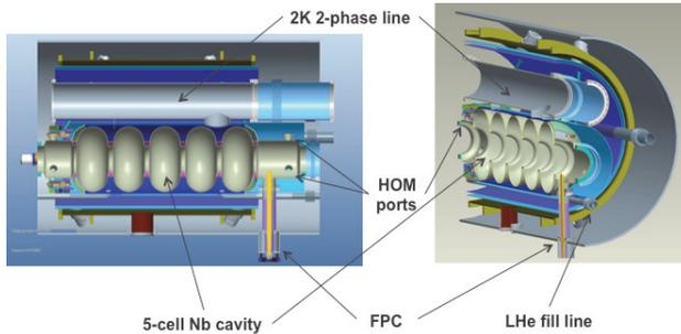
Figure 3: Preliminary layout of a cryounit for eRHIC.
