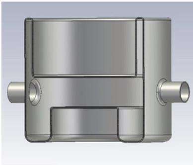
Figure 4: Concept model of QW crab cavity [12].
