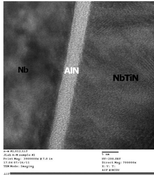
Figure 2: TEM image of a FIB cut NbTiN/AlN/Nb/Cu structure.
