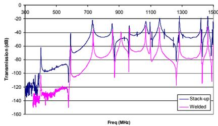
Figure 7: Preliminary RF measurements of cavity before final EB welding in the stack-up configuration, and measurements of welded cavity after final weld.
