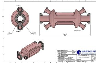
Figure 9: 750 MHz crabbing cavity design.
