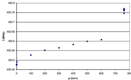
Figure 8: Finished cavity leak-check and final round of room temperature RF measurements.
