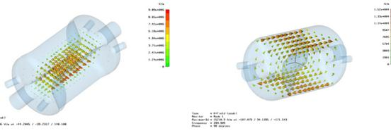
Figure 3: Electric (left) and magnetic (right) field distribution in the improved parallel-bar deflecting structure for the operating fundamental mode.
