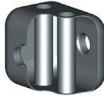
Figure 1: Concept of the parallel-bar deflecting structure.
