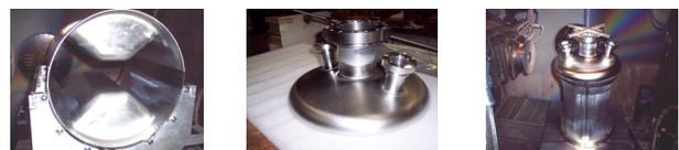
Figure 5: Crabbing cavity subassemblies (left and middle) and the full EB welded cavity (right).
