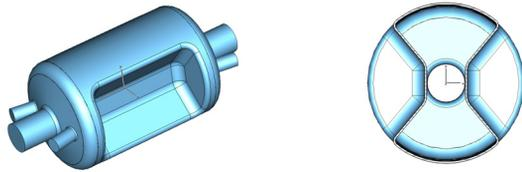
Figure 2: Improved parallel-bar deflecting structure.
