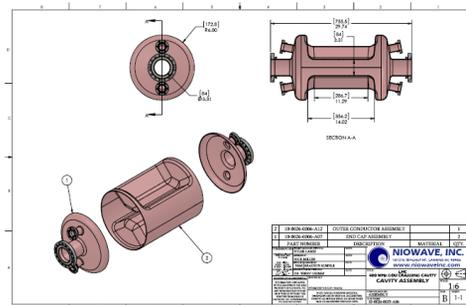
Figure 4: Final assembly mechanical drawing of the 400 MHz Crabbing cavity for LHC HiLumi Upgrade.
