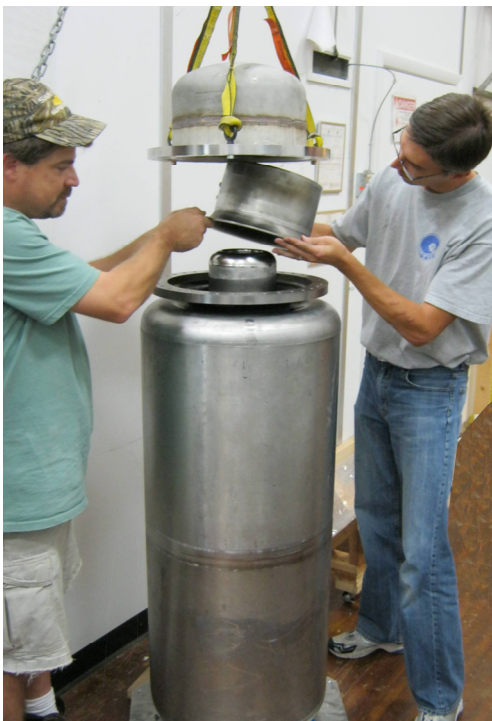
Figure 4: Three main cavity subassemblies shown before final electron-beam welding (above) and the welded cavity shown being fit with a niobium test head and stainless steel vacuum head for initial RF measurements and testing (below).
