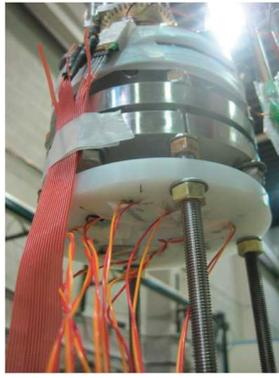
Figure 5: TE cavity sample plate thermometry system.
