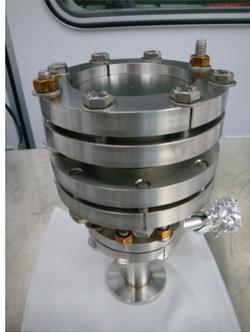
Figure 2: The TE pillbox cavity with SS316 flanges and pumping adapter tubes.
