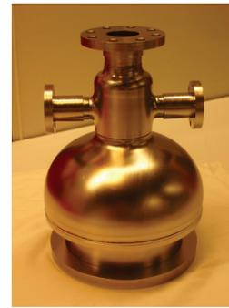
Figure 3: TE mushroom cavity after a heavy BCP.
