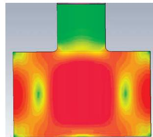
Figure 1: Magnetic field contour plot of the TE<sub>011</sub> mode of TE pillbox cavity. Red color indicates higher magnetic field region.
