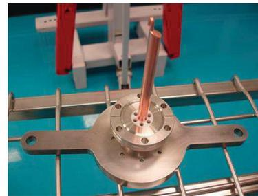
Figure 4: An off-center hook coupler for TE sample cavity test.
