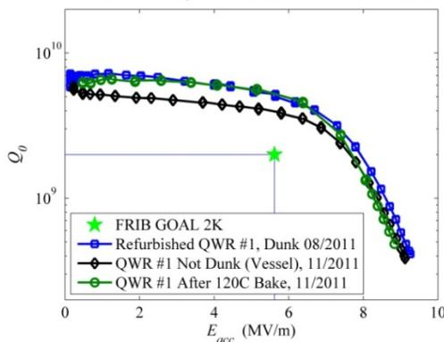
Figure 7: 2K comparisons of dunk test and the vertical cryostat configuration and again after a 120 C bake.
