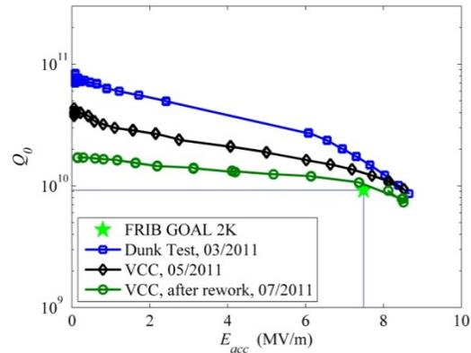
Figure 5: Sequential vertical tests of a FRIB HWR, dunk test, helium vessel test, then after a helium vessel rework.
