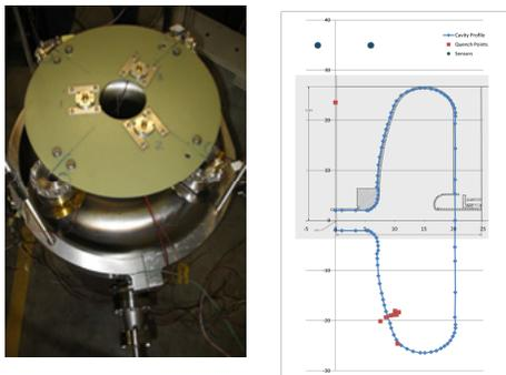
Figure 3: Quench detection set-up (left) and results from second sound (right).
