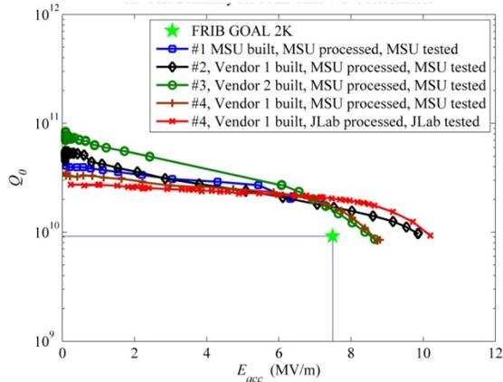
Figure 2: HWR Dunk Test Results.
