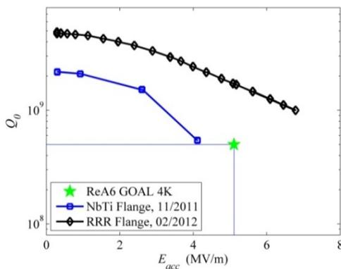
Figure 6: QWR niobium versus NbTi bottom flange results.
