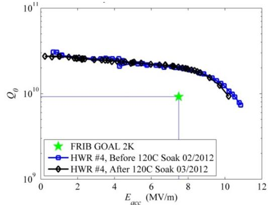
Figure 4: HWR low temperature bake performed at JLAB.
