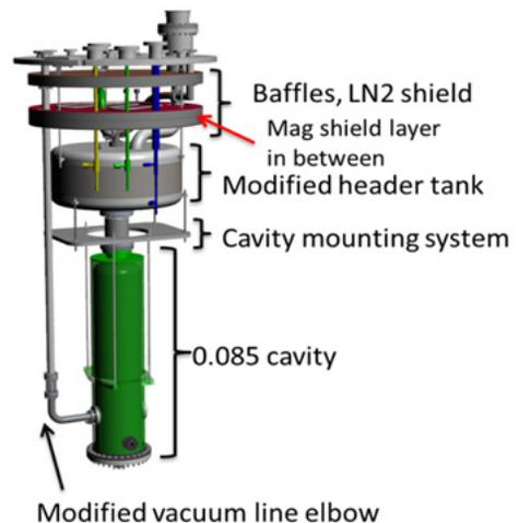
Figure 1: FRIB vertical test Dewar insert for ( $\beta=0.085$  QWR shown); The insert can adapt to hold both ReA and FRIB QWRs and FRIB HWRs.
