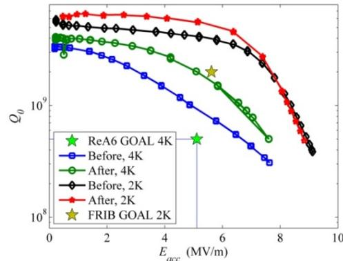
Figure 8: 4K and 2K comparison of the 120 °C for 48 HRs low temperature bake.
