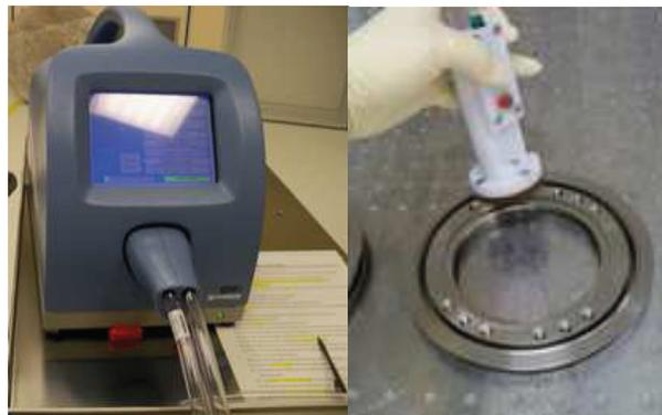
Figure 1: QIII+ surface particle counter and 2" probe scanning titanium blind tapped holes flange.
