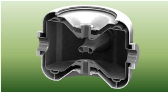
Figure 1: The mechanical design of SSR1 of 3<sup>rd</sup> generation. A transition ring couples the niobium cavity wall to the steel vessel wall and can be seen at the bottom. The bellows is visible at the top. The niobium components are rendered in dark grey, the stainless steel ones are rendered in light grey.
