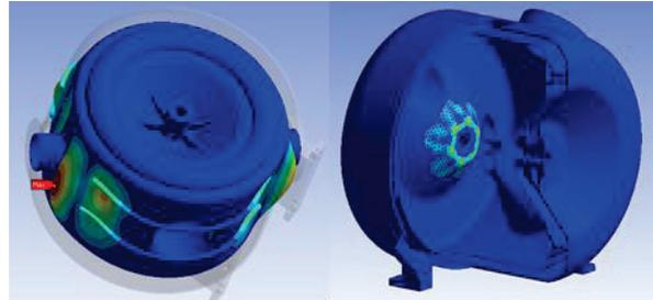
Figure 3 : Results of the buckling analysis (left) showing the area of failure next to one of the coupler ports and plastic collapse analysis (right) showing the area of failure at the base of the beam pipe ribs.
