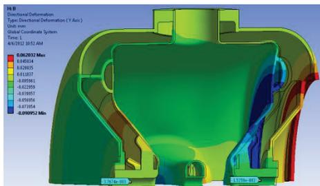
Figure 2 : Results of a coupled analysis to evaluate the  $df/dp$  of the proposed design. Despite the non-negligible deformations up to 90 microns (blue areas), the  $df/dp$  of the cavity results being close to zero in virtue of the aforementioned compensation approach.
