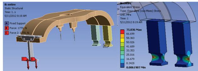
Figure 6 : Load case with  $F = 2 \times 1770$  N and springs mimicking the cavity at the probe ends (left) and stresses in the joint (right) topping at 75 MPa.
