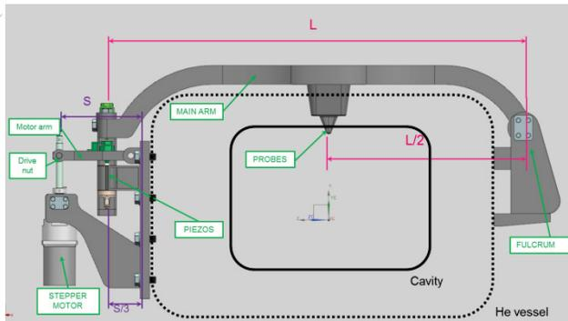
Figure 4 : SSR tuner scheme. The mechanical advantages are about 2:1 between piezos and probes, and about 3:1 between motor and piezos.
