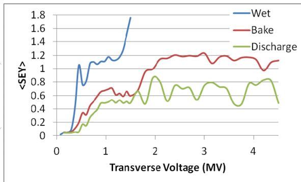
Figure 3:  $\langle \text{SEY} \rangle$  versus transverse voltage for three different surface emission models.
