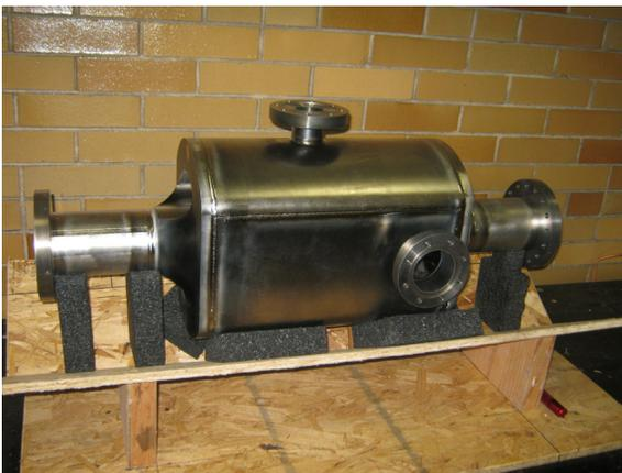
Figure 7: Manufactured Niobium cavity at Niowave.
