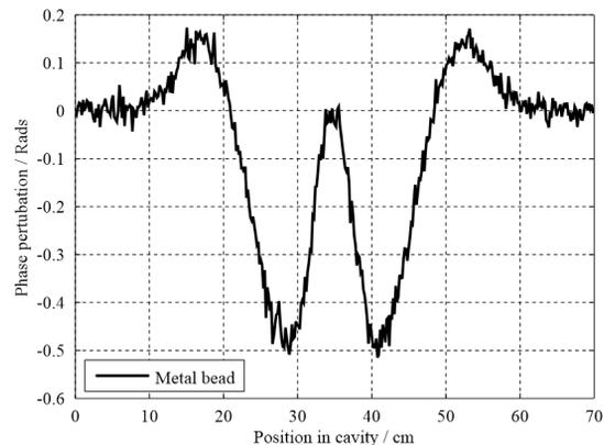
Figure 1: Bead-pull measurement of cavity phase shift versus longitudinal "bead" position
