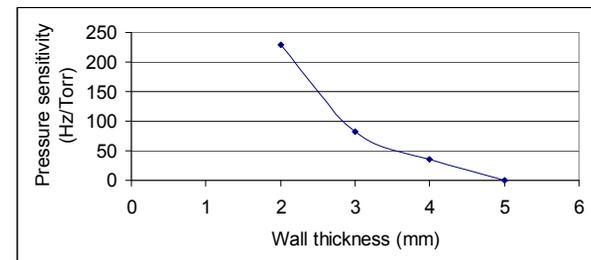
Figure 5: Pressure sensitivity of the cavity versus wall thickness.
