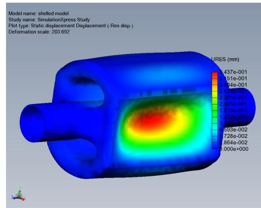
Figure 4: Cavity deformation due to atmospheric pressure difference.
