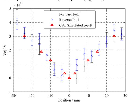
Figure 2: Measured longitudinal voltage at 1 J stored energy from bead-pull versus offset of measurement.
