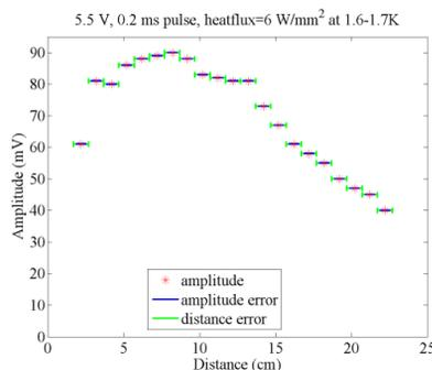
Figure 3: A distance variation measurement shows maximum amplitude detected by an OST at ~9 cm distance from the heater.
