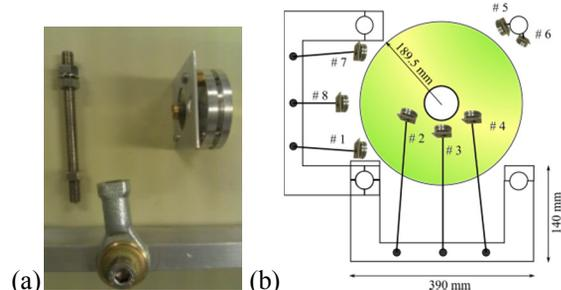
Figure 2: (a) The aluminium OST support can be mounted to a desired height and the three extensions holding their OSTs are adjustable towards the cavity (b) Three OSTs each govern  $1/4$  equator area and another  $1/4$  iris region respectively. Two OSTs are mounted on a rod supporting the cavity with # 5 facing the equator and #6 is 9.3 cm above #5.
