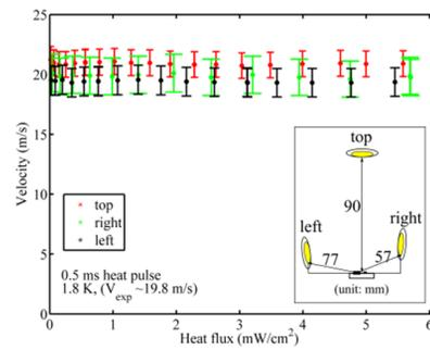
Figure 9: Response of OSTs at the top of the heater and two OSTs on the sides when power is increased to deliver to the heaters.
