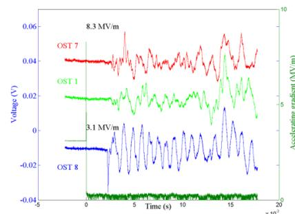
Figure 6: A quench detected by three OSTs.
