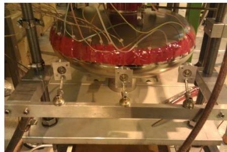
Figure 1: SMDs are distributed around the equator, iris and other surfaces corresponding to different OSTs as in Fig. 2(b).
