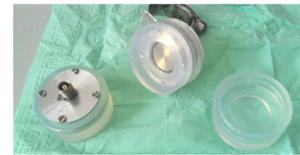
Figure 5: OST protection caps are made to protect membrane against damage or pollution during the mounting process.
