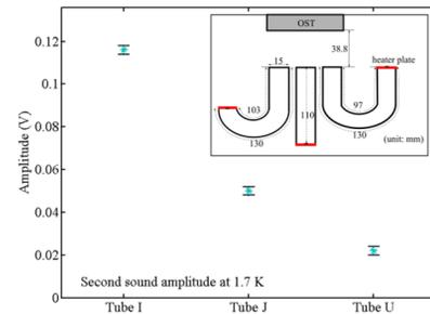
Figure 4: Second sound is detected with amplitude attenuation through tubes having bent structure.
