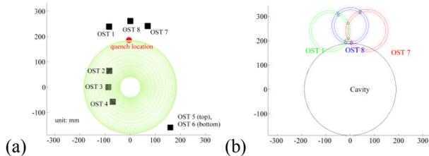
Figure 8: Quench localisation by using a minimisation method (a) and (b) intersection area using a 30 m/s parameter retrieved from the minimisation method.
