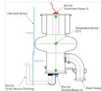
Figure 2: Setup for vertical test.
