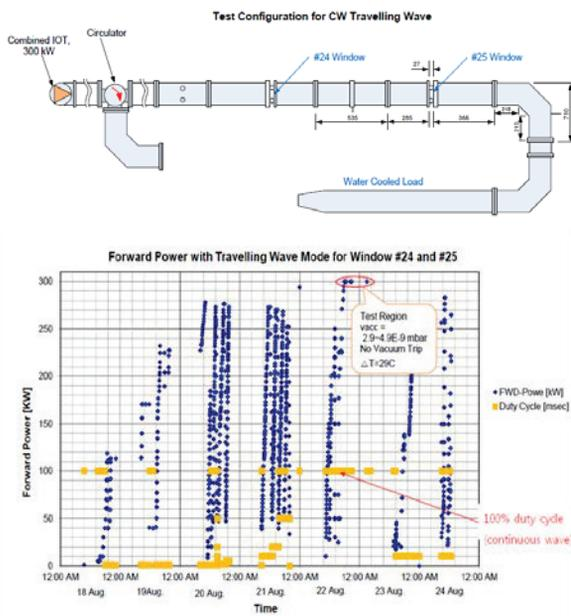
Figure 4: Test setup (upper) and processing history for TW mode (lower).
