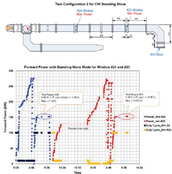
Figure 5: Test setup (upper) and processing history for SW mode (lower).
