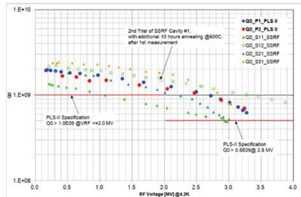
Figure 3: Measured cavities' performance, Eacc vs  $Q_0$ .
