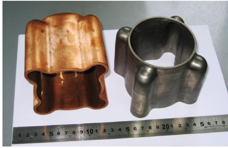
Figure 4: Scaled OFHC prototype and fabricated niobium seamless fluted beam pipe.
