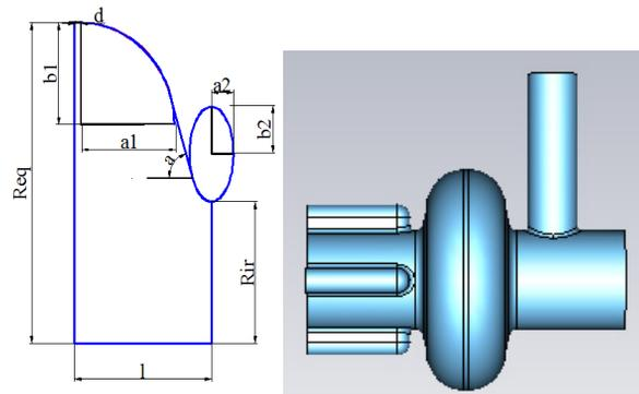
Figure 3: Cell shape and CST model of the new type single cell cavity.
