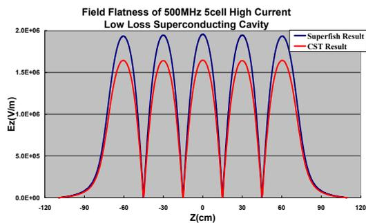
Figure 5: 500MHz 5cell cavity model by CST and field flatness output of CST and Superfish.
