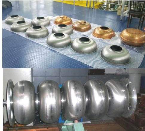
Figure 6: The pressed niobium half cells, copper half cells and EBWed cavity.
