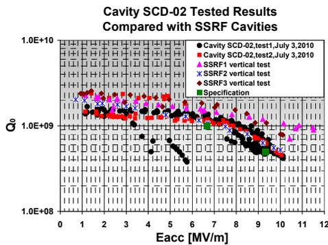
Figure 2: Vertical test results of the 500MHz single cell superconducting cavity fabricated, surface prepared at SINAP, compared with those of the superconducting cavities installed in SSRF storage ring.
