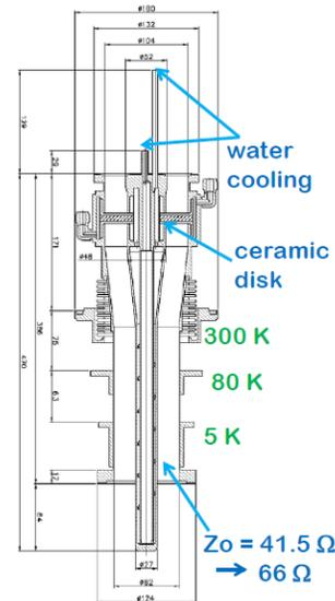
Figure 2: Schematic drawing of CW input coupler with coaxial ceramic RF window.
