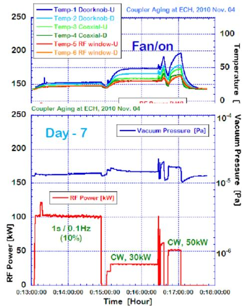
Figure 5: RF conditioning results of #1 and #2 prototype input couplers: temperature rises (top), vacuum pressure (middle) and input RF power (bottom).
