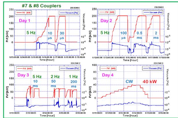
Figure 9: RF conditioning procedure of #7 and #8 input couplers for four days (maximum CW 40 kW): input RF power (red line) and vacuum pressure (blue line).
