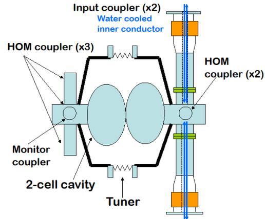
Figure 1: Conceptual structure of 2-cell cavity with 2 input couplers and 5 HOM couplers for cERL injector.
