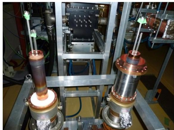
Figure 6: Surface colour change by excessive heat-up around bellows of inner conductors in #1 and #2 prototype input couplers after conditioning at CW 50 kW for 30 minutes.
