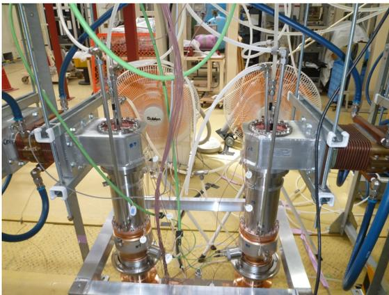
Figure 8: High power test stand for RF conditioning with improved cooling by nitrogen gas flow in a pair of #7 and #8 input couplers.
