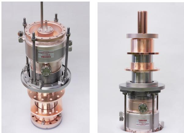
Figure 3: Two prototype input couplers, (#1 and #2).
