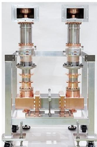
Figure 4: High power RF test system consisting of two input couplers, coupling waveguides as a vacuum chamber, coaxial lines and doorknob-type transitions.
