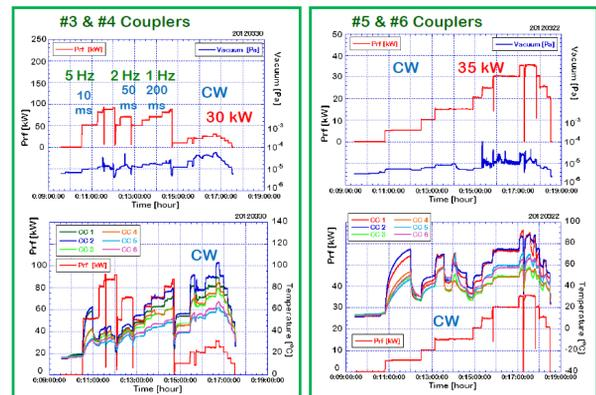
Figure 10: Temperature rises during conditioning in #3 and #4 input couplers (maximum CW 30 kW) and #5 and #6 input couplers (maximum CW 35 kW).
