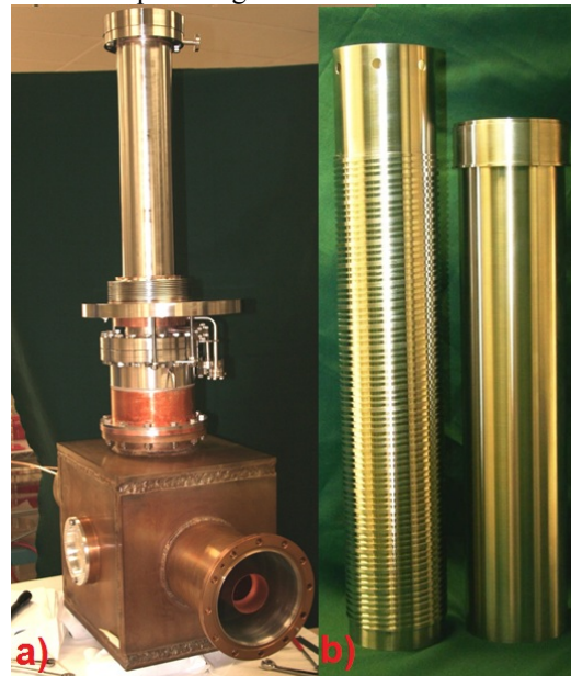
Figure 6: a) Power coupler prototype. b) GHe cooling inner wall (on the left) with engraved cooling channels and outer wall (on the right) with a smooth cylindrical shape.
