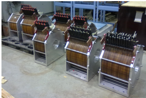
Figure 2: Completed GS1, GS2, CS1 and CS2 magnets.
