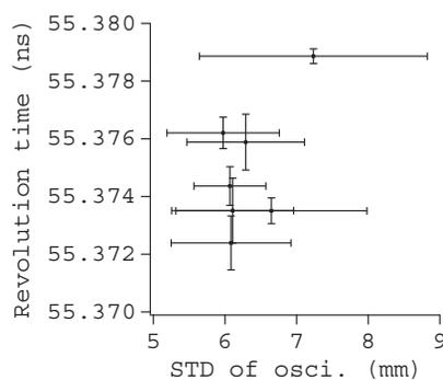
Figure 3: Dependence of bunch revolution time measured at a single BPM against the initial size of the coherent oscillation.
