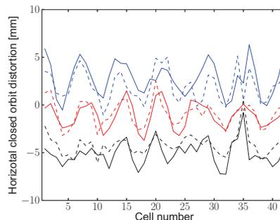
Figure 1: Comparison of measured residual horizontal COD (solid) after correction with predictions (dashed) at 14.3 MeV/c (black), 16.4 MeV/c (red) and 18 MeV/c (blue).
