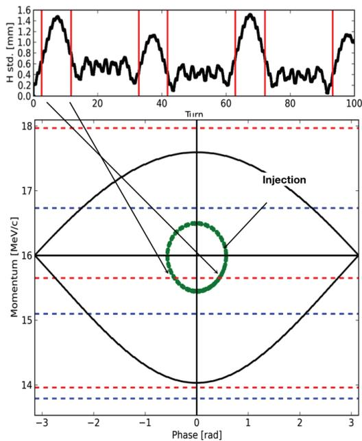
Figure 2: Slow resonance crossing near a stable fixed point during a synchrotron oscillation. Orbit growth is reversed.
