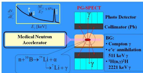
Figure 3: Principle of PG-SPECT.
