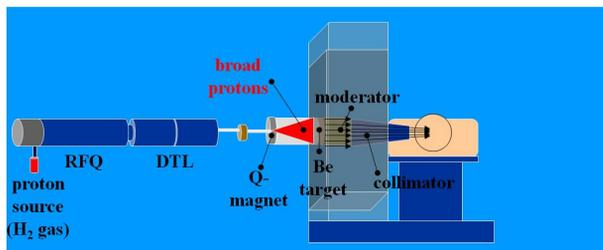
Figure 4: Layout of medical neutron accelerator at PMRC.
