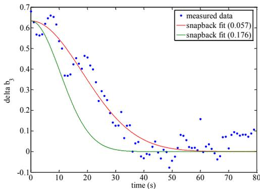
Figure 2: Snapback of  $b_3$  at the beginning of the ramp.
