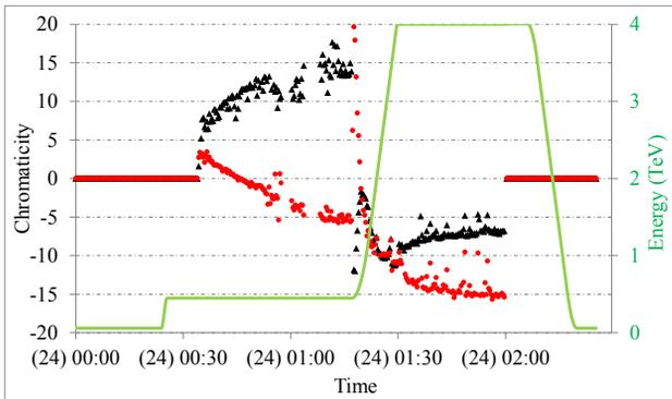
Figure 1: The bare ramp: chromaticity decay, snapback, drift during ramp and decay at 4 TeV.
