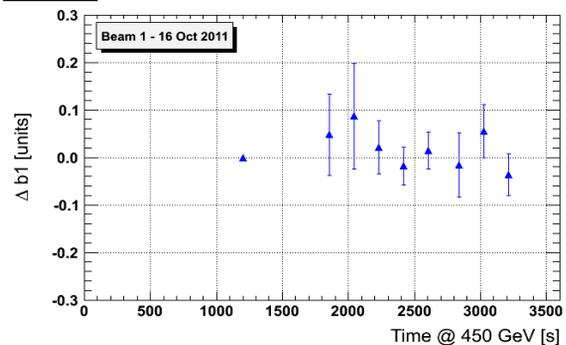
Figure 3: Estimate of decay of the dipole main field through beam measurements at injection.
