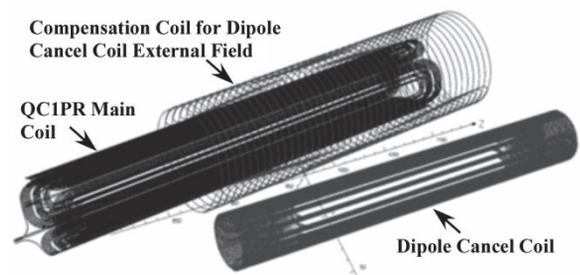
Figure 6: An integral field dipole cancel coil proposal.
