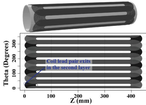
Figure 3: A Serpentine style coil winding example, the dual layer octupole pattern for QC2EL. Here the coil is wound using a continuous length of wire and the lead pair exits via an open ended pole in the second layer.
