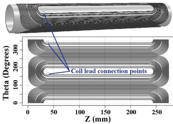
Figure 2: A planar pattern coil winding example, the single layer skew dipole pattern for QC1PL. Single layer planar coils have leads trapped at the poles.
