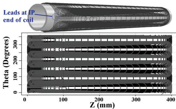
Figure 5: Example of lowest order,  $b_3$ , cancel coil pattern. The leads come out at the IP end of the magnet (same as for main coil). Non-lead end turn spacing is dramatically increased to make the sextupole gradient follow the desired cancel coil field fall-off profile.
