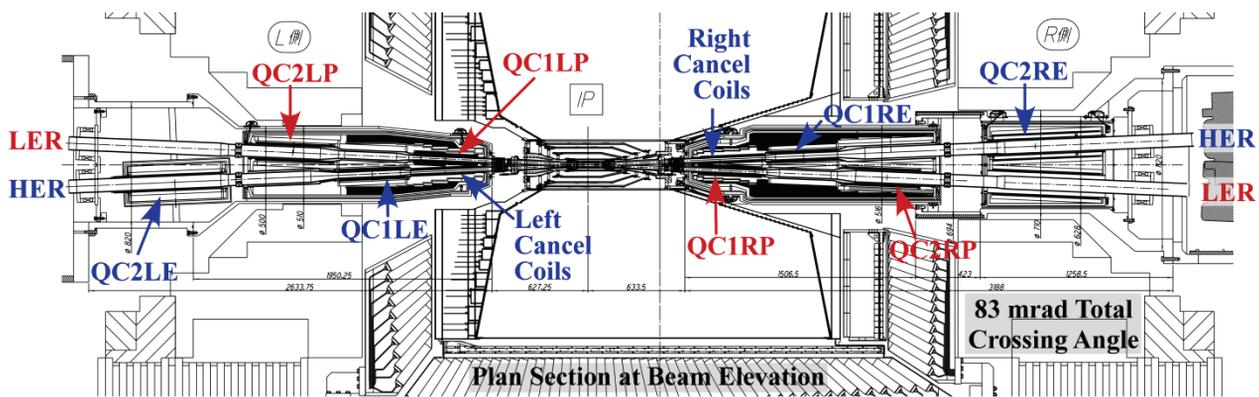
Figure 1: SuperKEKB IR layout inside Belle-II with high energy,  $e^-$ , (HER) and low energy,  $e^+$ , (LER) rings indicated.
