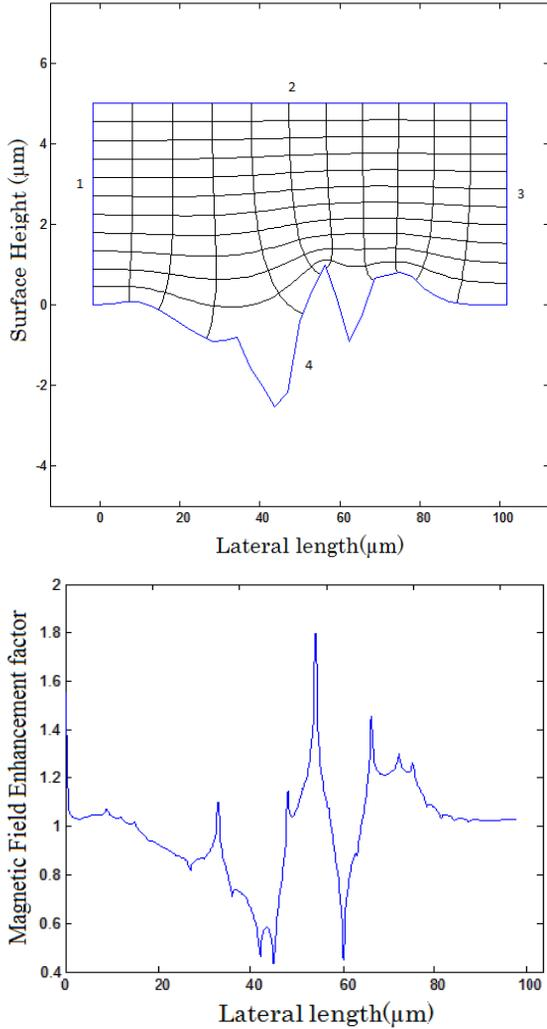
Figure 2: The Local Geometric Magnetic Field Enhancement factor (LGMFE) map along surface contour 4.
