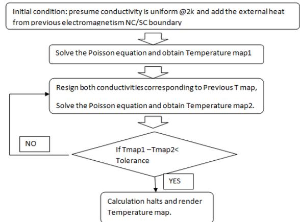
Figure 4: The flow chart of thermal equation simulation. With the electromagnetism output described in Fig. 4, one can calculate the temperature map across the cavity wall as demonstrated in figure below.
