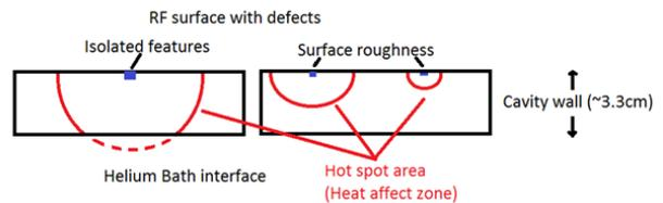
Figure 8: ‘Hotspot’ comparison between isolated and homogeneous surface features. The blue areas are geometric defects, while red circle suggests the ‘heat affected zone’.
