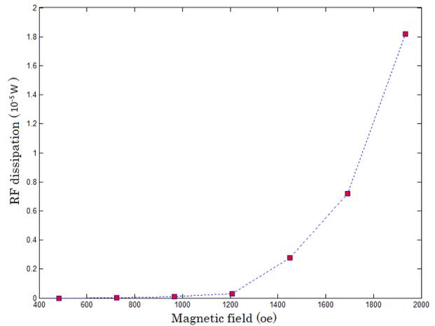
Figure 7: The integrated RF loss vs external magnetic field.
