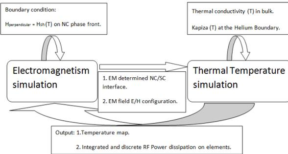
Figure 6: Flow chart of electromagnetism and temperature simulations.
