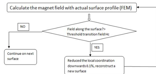
Figure 1: Flow chart to calculate E/M field configuration.
