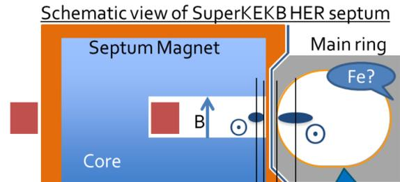
Figure 4: The schematic view of the SuperKEKB septum is shown.
