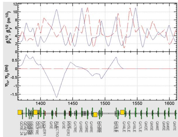
Figure 6: The result of optics study is shown. The top and middle rows indicate  $\beta_R$  and  $\eta_R$ , the blue and red color represent the horizontal  $x$  and vertical  $y$  axes, respectively. The bottom part shows a part of a number of magnets on the beam line. The injection point is named as 'INJECTIO', where  $\eta_{xR}$  takes the minimum.
