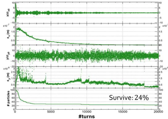
Figure 1: The tracking example of the betatron injection are shown. From above, the horizontal beam spread  $x/\sigma_{x0}$ , the horizontal emittance  $\varepsilon_x$ , the vertical beam spread  $y/\sigma_{y0}$ , the vertical emittance  $\varepsilon_y$  and the number of surviving particles are represented as the function of the number of turns.
