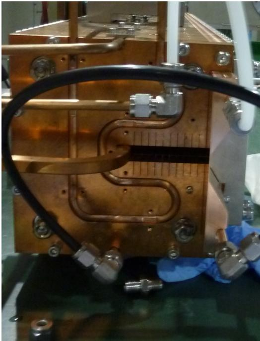
Figure 5: The picture of septum magnet is shown. The direction of view is the longitudinal along the beam line. The septum conductor is seen in the right-side of the core gap which is the pass for the injected beam; a vacuum duct for stored beam is placed on the right-side of the septum magnet.
