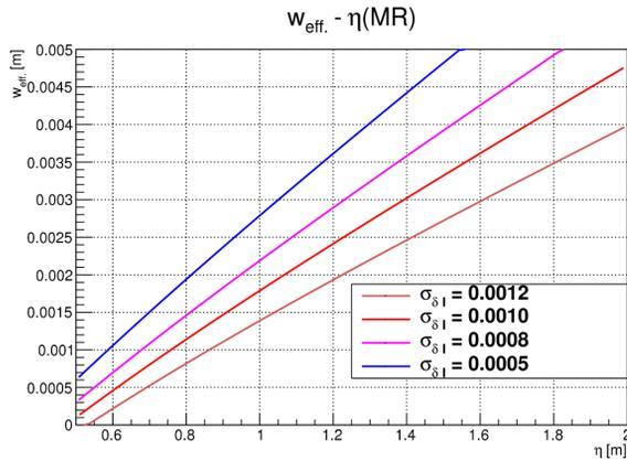
Figure 3: The allowed  $w_S$  to the horizontal dispersion on some cases of energy spread.
