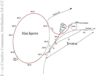
Figure 1: The Fermilab accelerator complex. The path of protons from the Booster synchrotron to the Antiproton Source Rings is shown in red.
