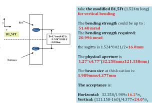
Figure 6: Acceptance of the vertical bending magnet.
