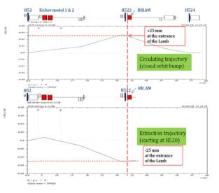
Figure 4: Trajectories of the circulating and extracted beam upstream of the Recycler extraction Lambertson.
