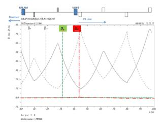
Figure 3: The Beta functions and dispersions of the new transfer line.
