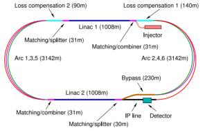
Figure 1: LHeC energy recovery linac configuration.
