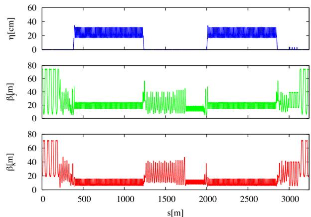
Figure 2: Damping ring lattice functions. From left extraction, arc, phase trombone, RF, wigglers, arc, circumference chicane, and injection.
