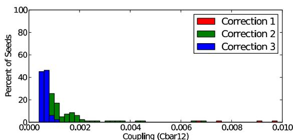
Figure 3: Histogram of the vertical emittance(top) and rms coupling ( $\overline{C}_{12}$ )(bottom) at the conclusion of each step in the low emittance tuning procedure for 100 lattice files with randomly chosen misalignments and multipole errors.
