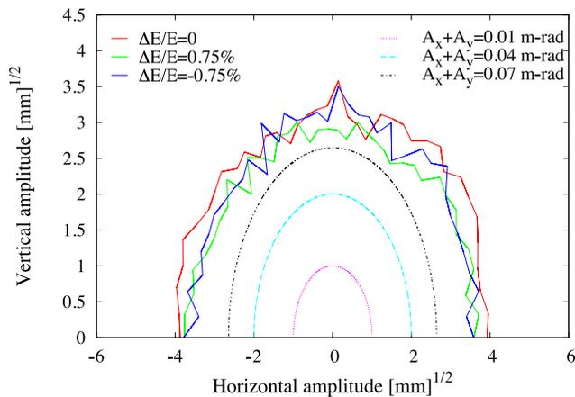
Figure 4: Dynamic aperture including multipoles, wiggler nonlinearities and magnet misalignments. Defined as the largest stable amplitude after tracking 1000 turns.
