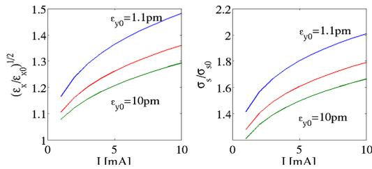
Figure 5: IBS growth versus current in the horizontal emittance (left) and in bunch length (right), at 1.6 GeV, for different equilibrium vertical emittance values.
