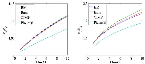
Figure 1: The IBS effect at the horizontal plane as calculated by Piwinski, B-M, Bane and CIMP at the nominal (left) and low energy (right) of the SLS.
