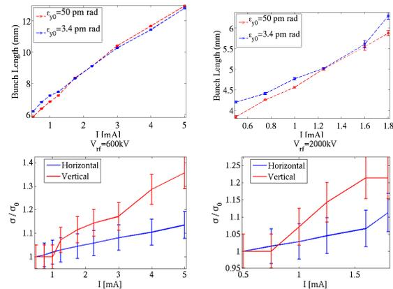
Figure 6: Left: Bunch length (top) and transverse beam size (bottom) data versus current for RF voltages of 600kV (left) and 2000kV (right).
