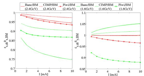
Figure 2: Horizontal (left) and vertical (right) emittance ratios for IBS models with respect to the BM method for nominal (red) and low energy (green) for different bunch currents.
