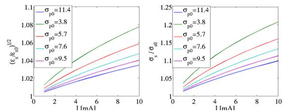
Figure 4: The IBS effect versus current in the horizontal emittance (left) and bunch length (right), for different equilibrium bunch lengths, at nominal energy.
