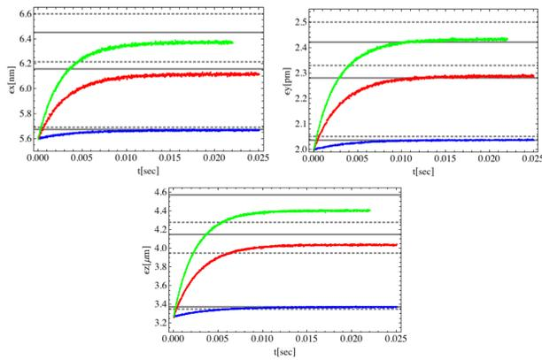
Figure 3: Evolution of horizontal (top, left), vertical (top, right), and longitudinal (bottom, left) emittances under the influence of IBS as obtained by the tracking code for different values of the bunch population:  $6 \times 10^9$  (blue),  $60 \times 10^9$  (red) and  $100 \times 10^9$  (green). Horizontal lines represent the steady state values predicted by Piwinski (full) and Bane (dashed) models for the considered bunch populations.
