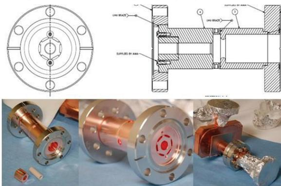
Figure 2: Top: mechanical drawing of the developed SW DLA structure; Bottom: finished structure.
