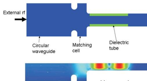
Figure 1: Top: 2D drawing of the developed SW DLA structure; Bottom: simulated E-field.
