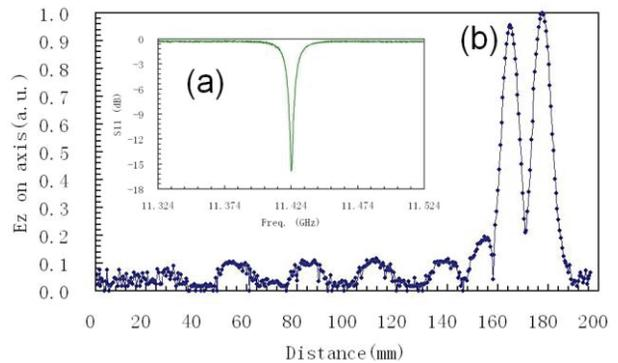
Figure 3: a): The measured S11 curve of the SW DLA structure; b): the bead-pull measurement results.
