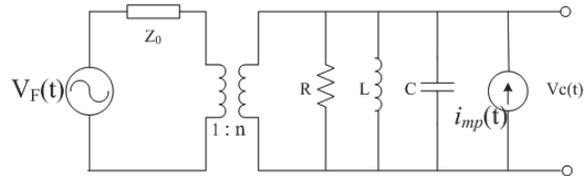
Figure 5: A simplified circuit model to represent a SW DLA structure with the multipactor loading current.
