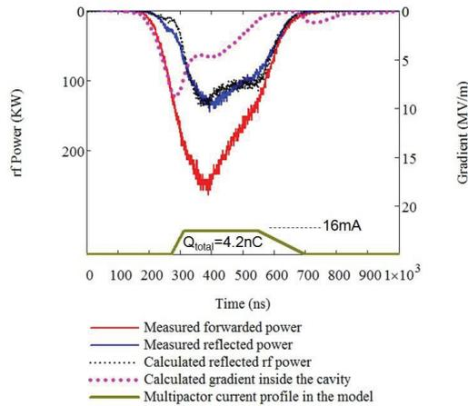
Figure 4: Comparison of the measured and calculated signals under dielectric multipactoring.
