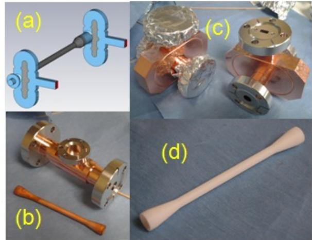
Figure 3. a) Design of the 26 GHz short pulse dielectric accelerator; b) Dielectric accelerator and metallized alumina tube; c) Two 26 GHz couplers; d) The alumina tube prior to metallization.
