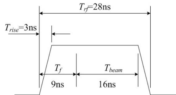
Figure 1. The 26 GHz rf pulse envelope for the short pulse TBA concept. A broadband and high group velocity ( $10\%c$ ) structure is needed for the fast rf rise and filling time.
