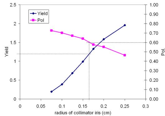
Figure 2: Yield and polarization as functions of photon collimator iris. 231m long RDR undulator driven by 150GeV electron beam. Flux concentrator of 14cm long and with ~3.5T peak field used as OMD.
