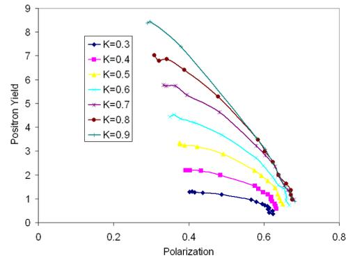
Figure 6: Yield vs polarization for undulator based positron source driving by 250GeV electron beam using undulator with different K and period of 1.15cm.
