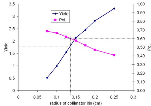
Figure 3: Yield and Polarization of 231m long RDR undulator driving with 175GeV beam. FC is used as OMD.
