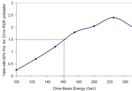
Figure 5: Yield associated with 60% polarization. 231m long RDR undulator with varying drive beam energy. Flux concentrator is used as OMD.
