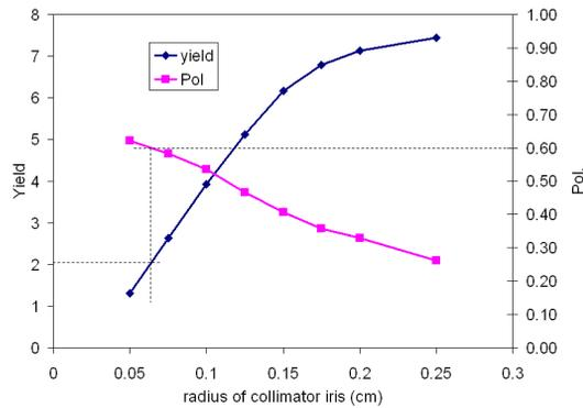
Figure 4: Yield and polarization of 231m long RDR undulator with 250GeV drive electron beam. FC is used as OMD.
