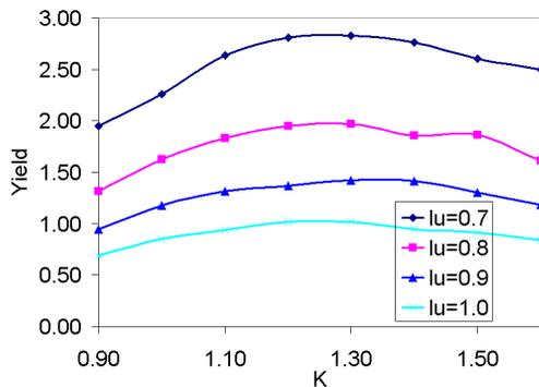
Figure 3: Results of undulator parameter scan for ILC positron source at 100GeV drive beam.
