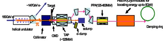
Figure 1: Positron source conceptual layout.
