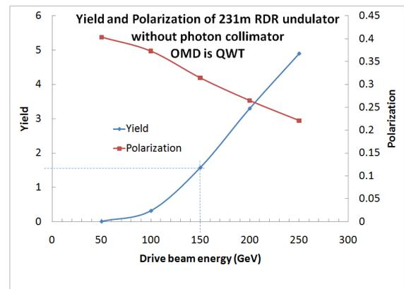
Figure 2: Yield and Polarization of RDR positron source with different drive beam energy.
