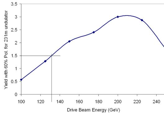
Figure 4: Yield with 60% polarization for undulator with K=0.9 and λ<sub>u</sub>=0.9cm.
