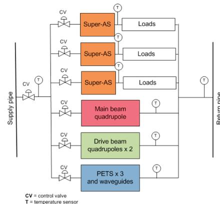
Figure 4 Cooling scheme for CLIC module type 1.
