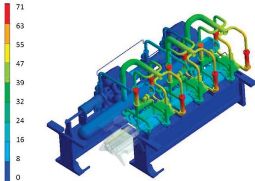
Figure 5 Deformed shape of CLIC module type 1 due to applied thermal RF loads (values in  $\mu\text{m}$ ).
