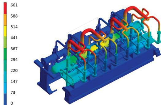
Figure 6 Deformed shape of prototype module type 0 due to applied thermal RF loads (values in  $\mu\text{m}$ ).
