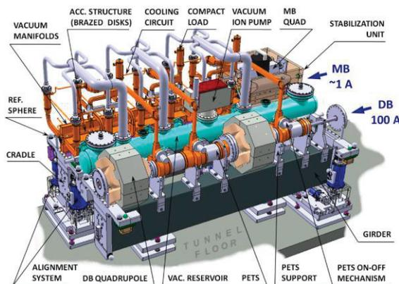
Figure 1 CLIC two-beam module typical configuration.
