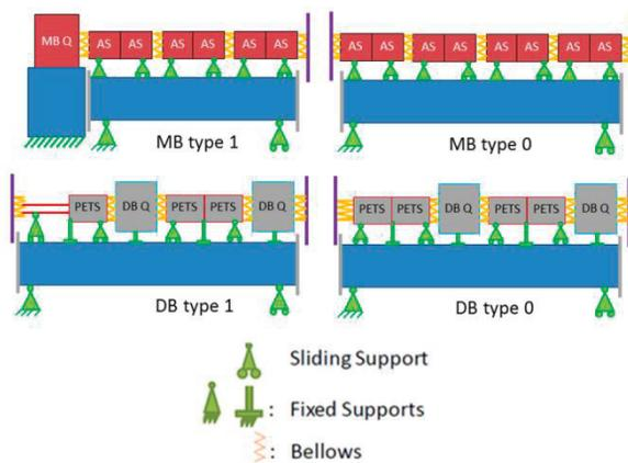
Figure 3 Constraints on the DB and MB girders for the CLIC modules type 1 and type 0.
