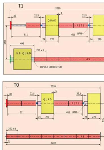
Figure 2 CLIC module scheme (T1 = type 1, T0 = type 0).
