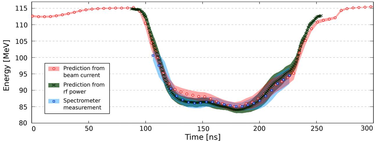
Figure 2: Beam energy along the pulse as measured in the spectrometer, and predicted from the beam current and the rf power. The symbols show the mean values over 48 pulses, while the bands show one standard deviation on each side.
