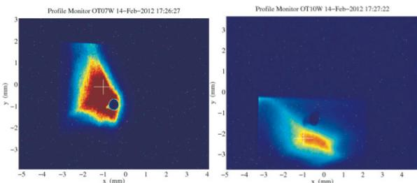
Figure 5: Electron beam spots at wiggler entry (left) and exit (right) flags. White crosshairs are the optical axis.
