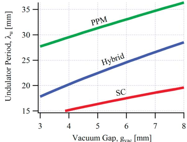
Figure 2: Qualitative examples of magnetostatic devices assuming  $K_{max} = 2.6$ . PPM refers to no-iron Pure Permanent Magnet; Hybrid to PPM + Fe poles; and SC to superconducting [11].
