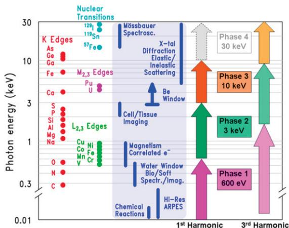
Figure 1: The blue area highlights techniques and science enabled at different energies; the right-hand side depicts the photon energies that can be reached with each construction phase. Further phases are possible.
