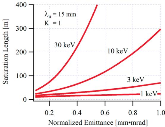
Figure 3: FEL saturation length vs. normalized emittance. The peak current is assumed to be 1 kA with an energy spread of 200 keV.
