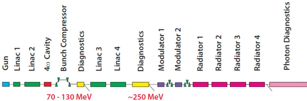
Figure 1: Schematic layout of CLARA. The overall length is ~80 m.
