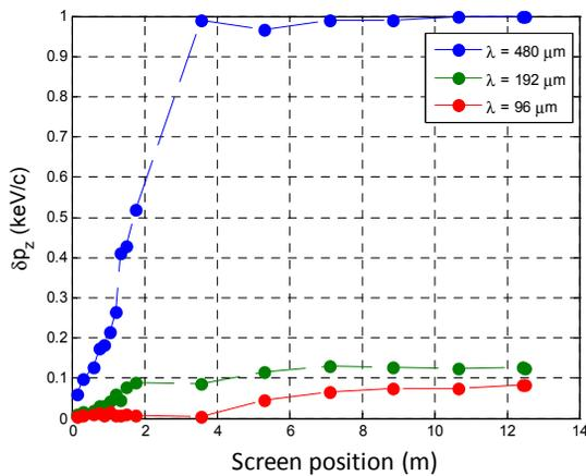
Figure 7: Amplitude of the momentum modulation along the low energy part.
