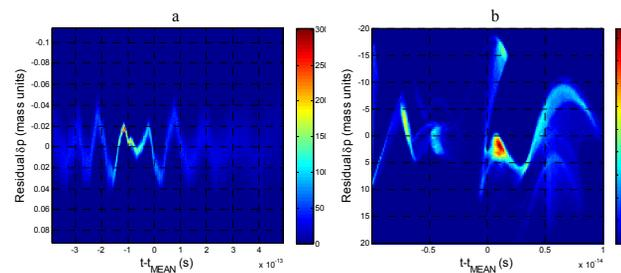
Figure 3: Start to end simulation. Residual momentum of the real shape bunch tracked to (a) the entrance of BC1 and (b) the Aramis undulators.
