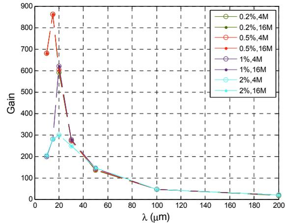
Figure 5: Spectral gain at the entrance of BC1 obtained by numerical simulations.
