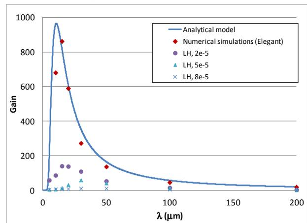
Figure 6: Comparison between the numerical simulation results and the analytical model at the exit of BC1. The results of the numerical simulations for several induced uncorrelated energy spread (laser heater) are also shown.
