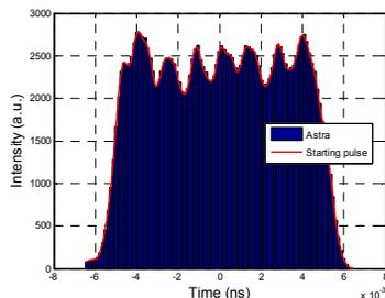
Figure 2: Temporal bunch profile at the cathode.
