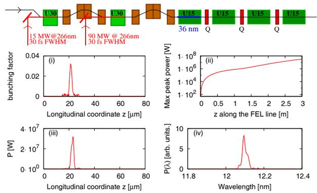
Figure 3: FEL at 12 nm in the EEHG configuration. (i) Bunching factor at the radiator entrance. (ii) Maximum peak power vs undulator radiator sections. Longitudinal (iii) power and (iv) spectral profile after 1 section of radiator. Seed: 30 fs-FWHM pulse with 15 MW and 88 MW peak power at 266 nm.
