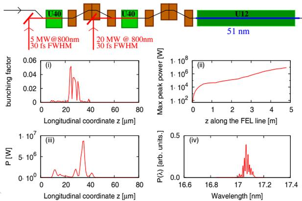
Figure 4: FEL at 17 nm in the EEHG configuration. (i) Bunching factor at the radiator entrance. (ii) Maximum peak power vs undulator radiator section. Longitudinal (iii) power and (iv) spectral profile after 1 section of radiators. Seed: 30 fs-FWHM pulse with 5 MW and 20 MW peak power at 800 nm.
