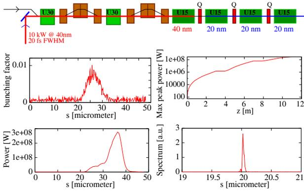
Figure 1: FEL at 20 nm in the HGHG configuration. (i) Bunching factor at the radiator entrance (ii) Power vs undulator radiator sections. Longitudinal (iii) power and (iv) spectral profile after the 4th radiator. Seed: 20 fs FWHM pulse with 10 kW peak power at 40 nm.
