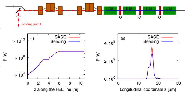
Figure 5: FEL performances at 400 MeV in SASE (red line) and Amplifier configuration (blue line)(seed power:1 kW), at 20 nm. (i) Output power along the radiator sections. (ii) Longitudinal power distribution at the exit of the second radiator. Electron bunch duration: 2 fs RMS, peak current: 10 kA, energy spread: $10^{-3}$ .
