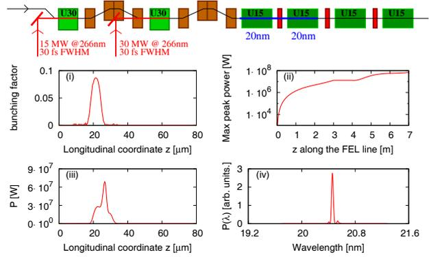
Figure 2: FEL at 20 nm in the EEHG configuration. (i) Bunching factor at the radiator entrance. (ii) Maximum peak power vs undulator radiator sections. Longitudinal (iii) power and (iv) spectral profile after 2 sections of radiators. Seed: 30 fs-FWHM pulse with 15 MW and 30 MW peak power at 266 nm.
