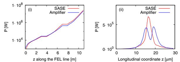
Figure 6: FEL performances at 400 MeV in SASE (red line) and Amplifier configuration (blue line)(seed power:1 kW). (i) Output power along the radiator sections. (ii) Longitudinal power distribution at the exit of the third radiator. Electron bunch duration: 20 fs RMS, peak current: 1 kA, energy spread:  $5 \times 10^{-3}$ .
