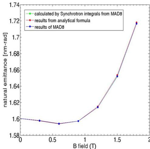
Figure 2: The dependence of TPS beam emittance on the W250 modulator wiggler field strength.
