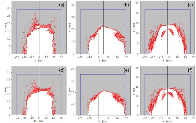
Figure 3: A comparison of TPS dynamic apertures calculated by using OPA with and without W250 wiggler. The subplots (a), (b) and (c) show the dynamic apertures of TPS bare lattice for 0%, +3.0% and -3.0% off energy particles respectively. Subplots (d), (e) and (f) show the dynamic apertures of TPS lattice with W250 operating at magnetic field strength of 0.92 T for 0%, +3.0% and -3.0% off energy particles respectively.
