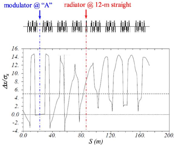
Figure 4: Calculated horizontal displacement of "satellite" bunch from core bunch with wiggler in position "A".
