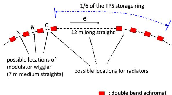
Figure 1: Possible locations of modulator wiggler and radiators in this evaluation study.
