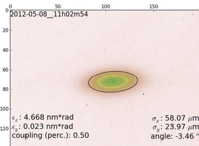
Figure 3: Emittance measurement.
