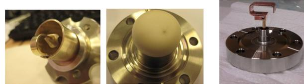
Figure 4: Cavity pick-up loops. The 2 pictures on the left correspond to the leaky old design. The picture on the right corresponds to the new in-vacuum design.
