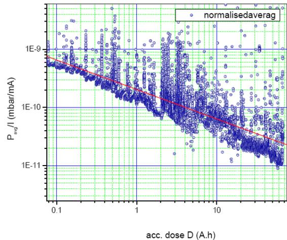
Figure 2: Normalised average pressure as a function of accumulated dose.
