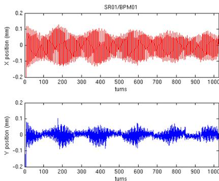
Figure 5: Residual orbit after adjustments.
