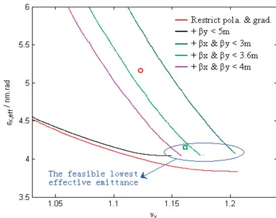
Figure 3: Optimal front of the effective emittance with beta function restrictions.
