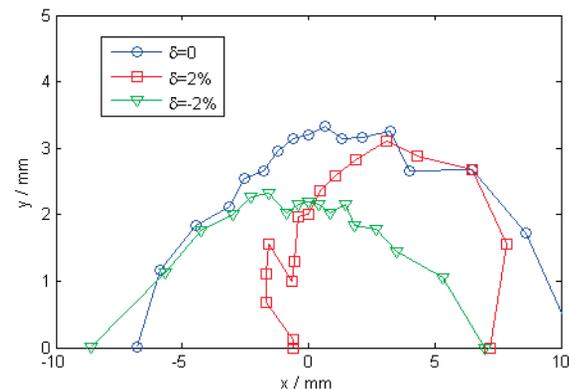
Figure 5: Dynamic apertures of the very low emittance optics, including on- and off-momentum particle.
