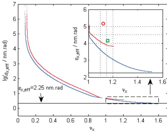
Figure 2: Optimal front of the beam emittance vs the horizontal tune per cell.
