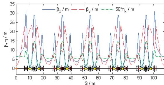
Figure 4: Linear optics in one super-period of the very low effective emittance optics.
