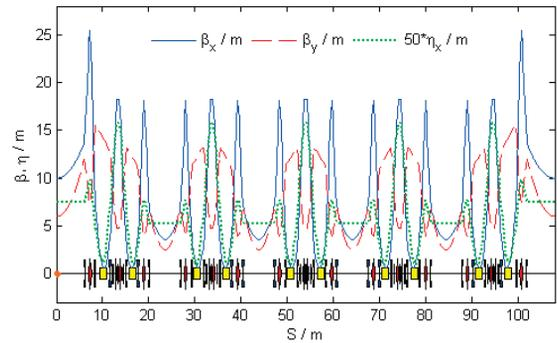
Figure 1: Nominal linear optics in SSRF.
