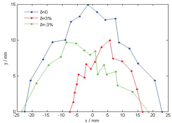
Figure 5: Dynamic apertures of the single-super bend lattice.
