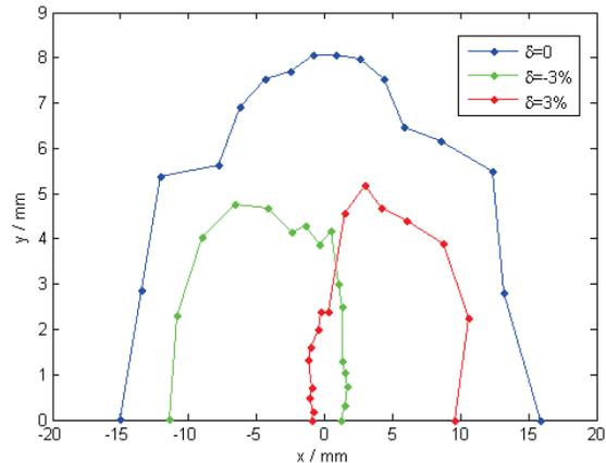
Figure 9: Dynamic apertures of the eight super bend lattice
