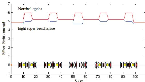
Figure 8: Horizontal effective emittance of the eight-super bend lattice and the nominal one.
