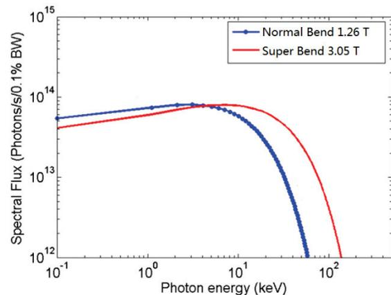
Figure 1: Photon spectrum of the normal bend and super bend in SSRF.
