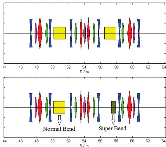
Figure 2: A single-super bend lattice compared to the nominal one.
