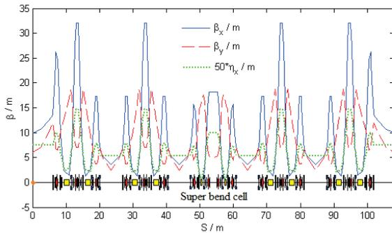
Figure 7: Linear optics in one superperiod.
