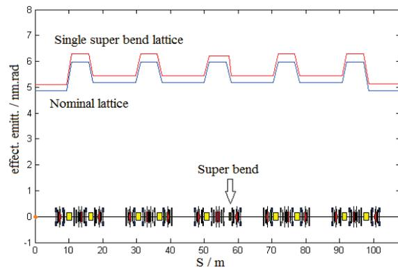
Figure 4: Horizontal effective emittance comparisons between the single-super bend and the nominal lattice.
