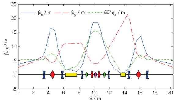
Figure 3: Linear optics in the cell with super bend
