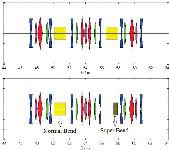
Figure 2: A single-super bend lattice compared to the nominal one.
