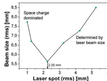
Figure 2: Optimized electron spot size vs laser spot size at the exit of the first solenoid after the gun. Below the laser spot size of 2.25 mm the beam size is increased by space charge effects (bunch charge 3 nC, laser pulse length 4 ps).
