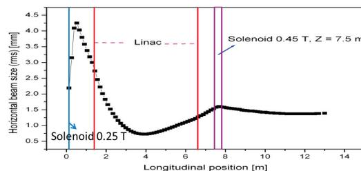
Figure 3: rms electron transverse beam size in FLUTE calculated with ASTRA between gun and chicane: bunch charge is 3 nC, laser pulse length 4 ps. Chicane magnets are set to zero current.
