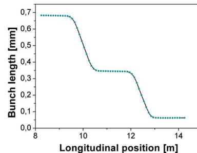
Figure 6: The development of the longitudinal bunch length in the bunch compressor tracked using a 3D space charge routine of ASTRA.
