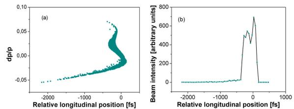
Figure 5: Compression of a 3 nC bunch calculated by a transfer matrix method ( $R_{56} = -40$  mm, bending radius is 3.4 m) (a) phase-space plot (b) bunch shape, the final rms longitudinal bunch length is 213 fs.
