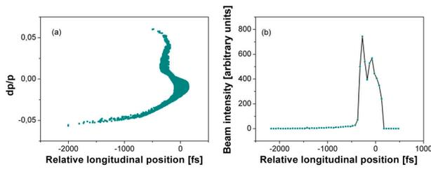
Figure 7: Simulations with ASTRA including the effect of space charge in the compressor: The phase space plot in (a) is similar to Fig. 5(a) and (b). The final rms longitudinal bunch length is 250 fs.
