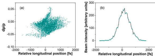
Figure 8: Influence of coherent synchrotron radiation and space charge effects on the final bunch shape. (a) phase space plot and (b) bunch shape, the final rms longitudinal bunch length is 419 fs
