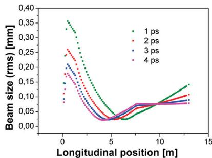
Figure 4: The rms transverse beam size for different laser pulse lengths. The bunch charge is 1 pC. Chicane magnets are switched off. The laser spot size at the cathode (0.05 mm rms) and solenoid (0.45 T) parameters are identical for all curves.
