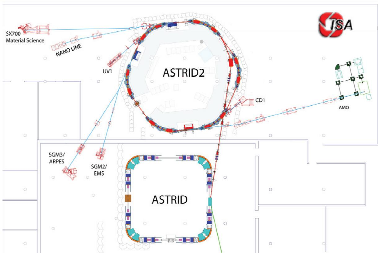
Figure 1: The transformed laboratory with the present storage ring ASTRID at the bottom, and the new light source ASTRID2 at the top. The existing beamlines on ASTRID will be upgraded and transferred to ASTRID2 together with new beamlines, which are named in the figure.
