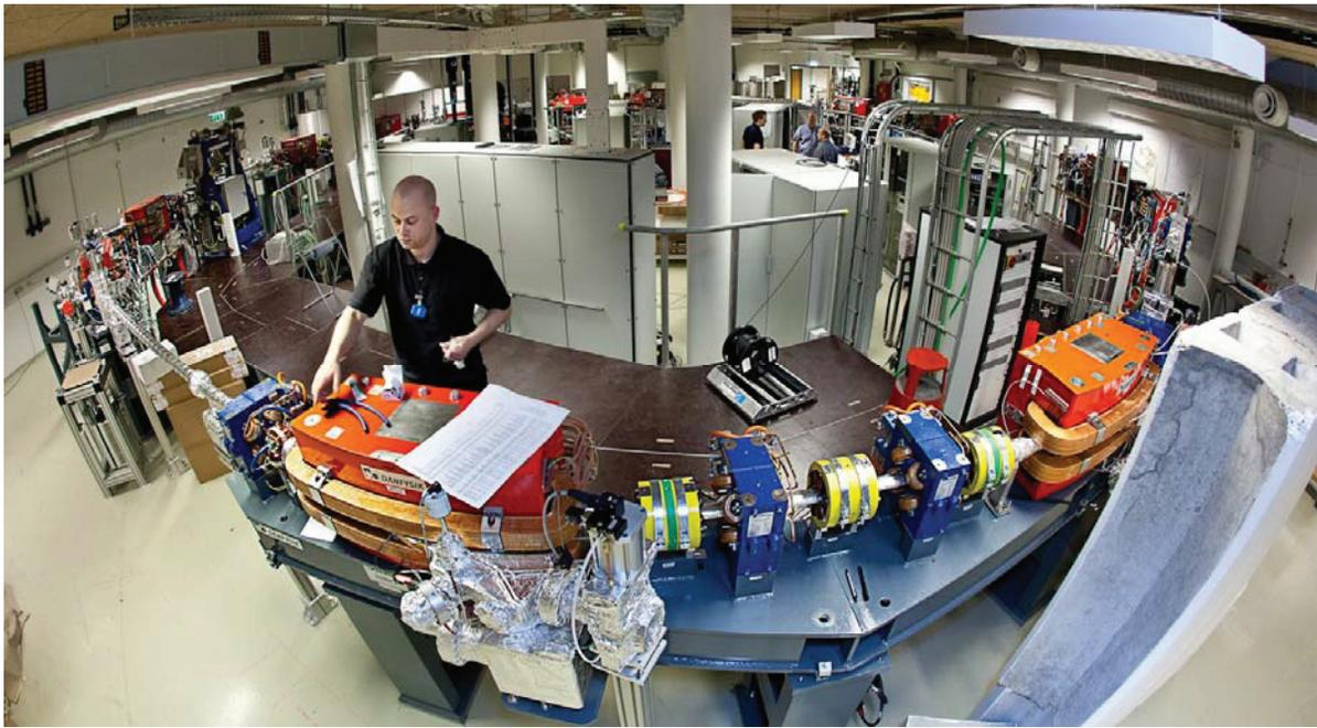
Figure 2: Close-up of the ASTRID2 ring with one of the six girders in the foreground showing the 2 red combined function dipole magnets, the blue quadrupole and the yellow sextupole magnets. The multi-pole wiggler is noticeable in the background. Power supplies etc. are seen in the centre of the ring.
