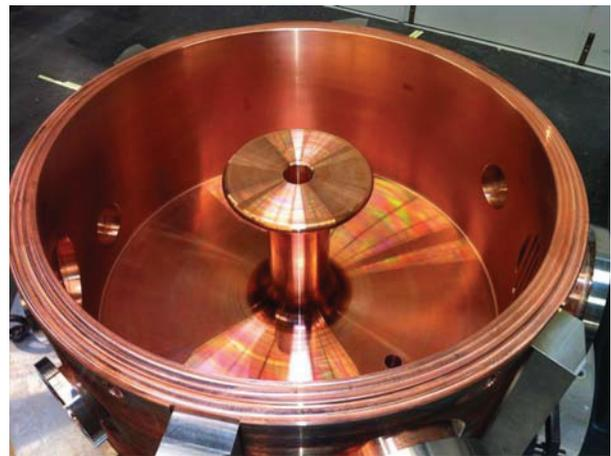
Figure 3: Inside of the 105 MHz ASTRID2 cavity before final weld of the endplate.
