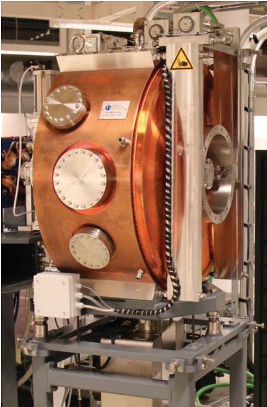
Figure 4: The 105 MHz ASTRID2 cavity mounted on its support stand. The mechanical tuning mechanism pulling on the right end-plate can be observed together with the gear on top.
