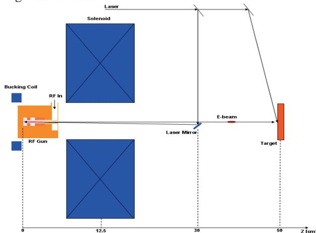
Figure 4: Schematic diagram of a proposed femtosecond electron diffraction experimental setup.
