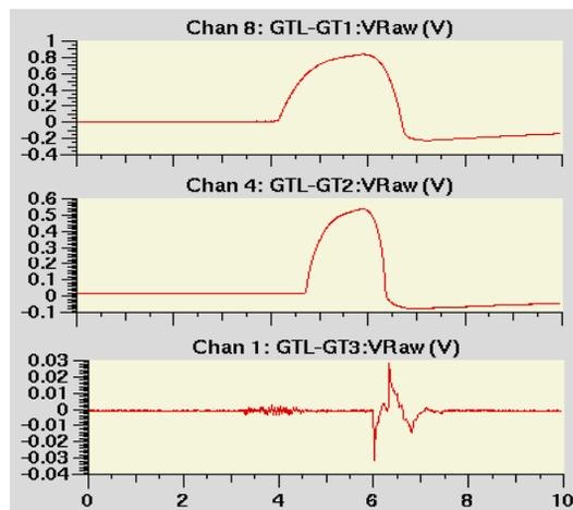
Figure 1: The electron bunch waveform in the Gun-to-Linac (GTL) transport line. Horizontal time axis in  $\mu$ s. Sensor voltage is converted to bunch charge, averaged over a 1 second period, and stored in the data acquisition system every 2 seconds.
