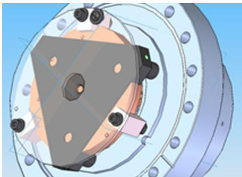
Figure 2: Photocathode assembly for QE measurements.
