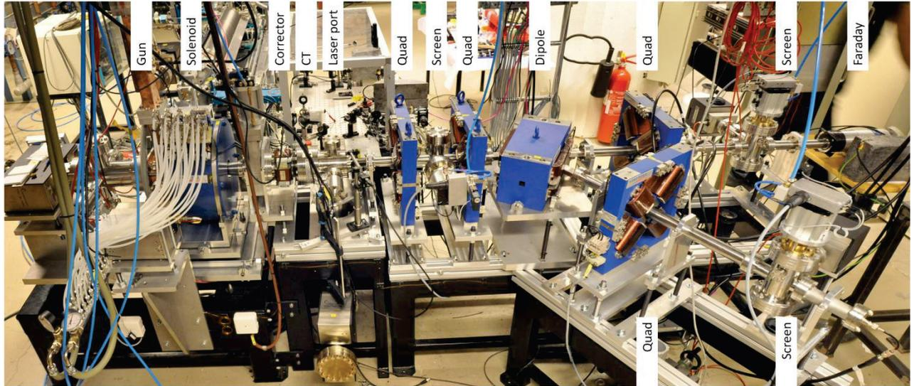
Figure 3: The MAX-lab gun test stand with the 1.6 cell RF gun and solenoid mounted.
