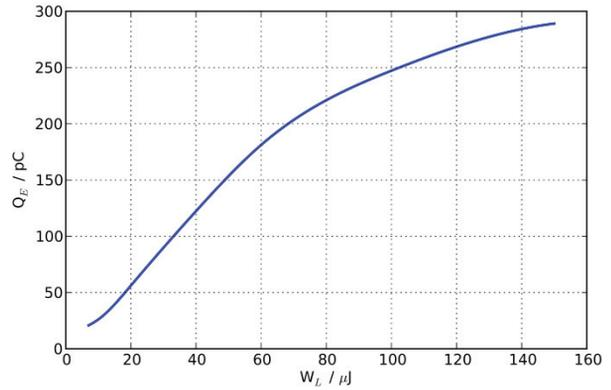
Figure 5: Emitted charge as a function of laser energy.
