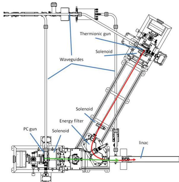
Figure 1: The MAX IV pre-injector layout with two RF guns injecting into the first linac.
